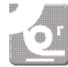
r mini = 8 D pendant la pose / during laying selon / according to EN 50565 (HD 516)
